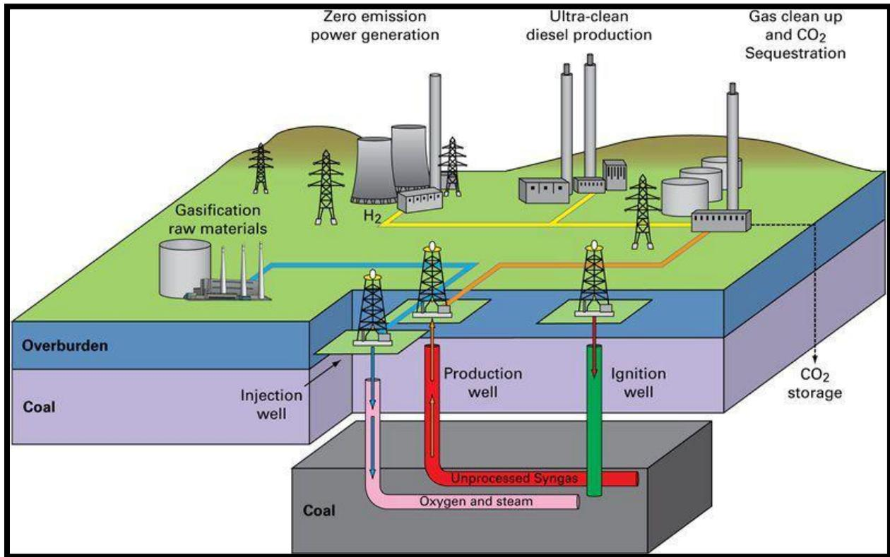
Fig: Underground Coal Gasification process.
